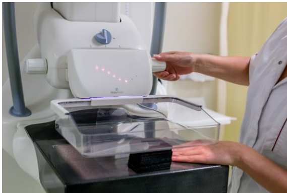
Picture of the Sensitive Sigma Paddle, when the target pressure (sixth LED) is reached.
